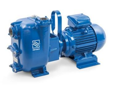
**Product Data** Suction port Threaded - 3" ISO 228 (BSP) Delivery port Threaded - 3" ISO 228 (BSP) Qmax 85 m<sup>3</sup>/h - 1416 l/min (374 USgpm) Hmax 35 m (115 ft) Solids handling 27 mm (1 ") Motor power 7,5 kW - 10 HP Motor type **IEC** standard Winding for inverters **Cast iron frame** Motor brand WEG W22 Premium Weight 140 ka
